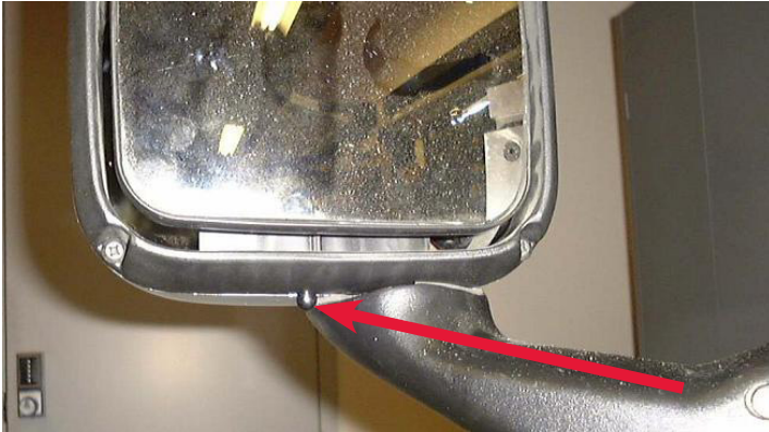
FIGURE 2-4: Aerodynamic Mirror OAT Sensor Location
